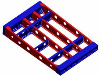
Wing Acoustic Box Internal Structure
