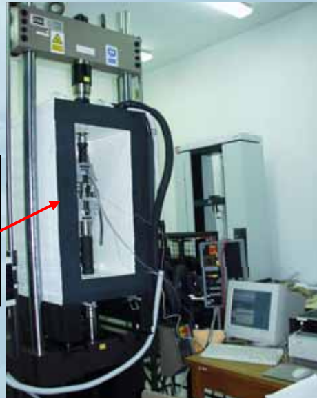
MTS device with a chamber for thermal conditioning
