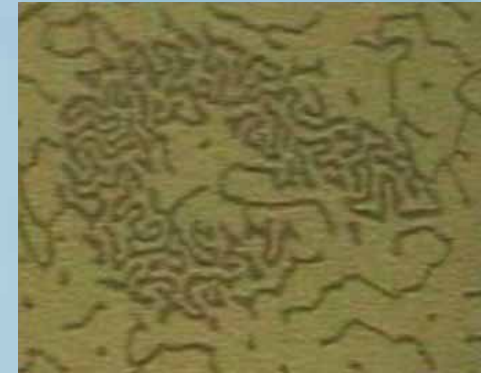
Magneto-Optic Crack Indication
