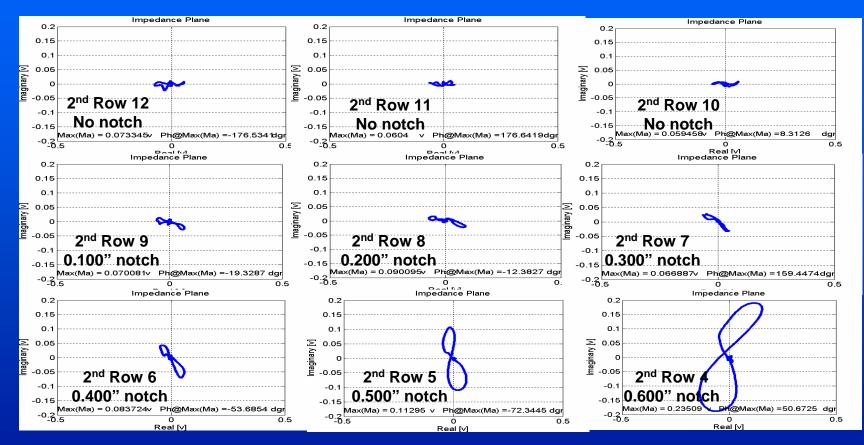
Note the immediate rotation of phase with the first EDM notch (0.100"), and the increasing phase rotation and amplitude with increasing notch size
