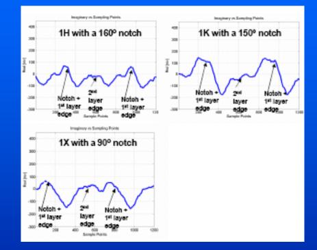
All the EDM notches are the same size. Variances in signals occur to the notch proximity to the 1<sup>st</sup> and 2<sup>nd</sup> layer edges. Note the increase in amplitude and increase in slope for the notched holes
