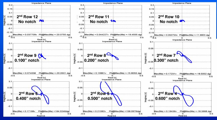
Again note the rotation of phase and increase in amplitude with increasing EDM size
