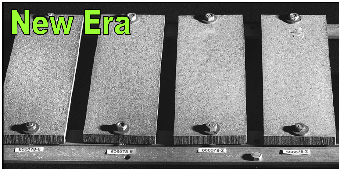
Al-Li 2099-type alloy w/ no coating exposed at seacoast for 14 yrs; No exfoliation occurred
