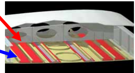
Strap Reinforced Integral Structure
