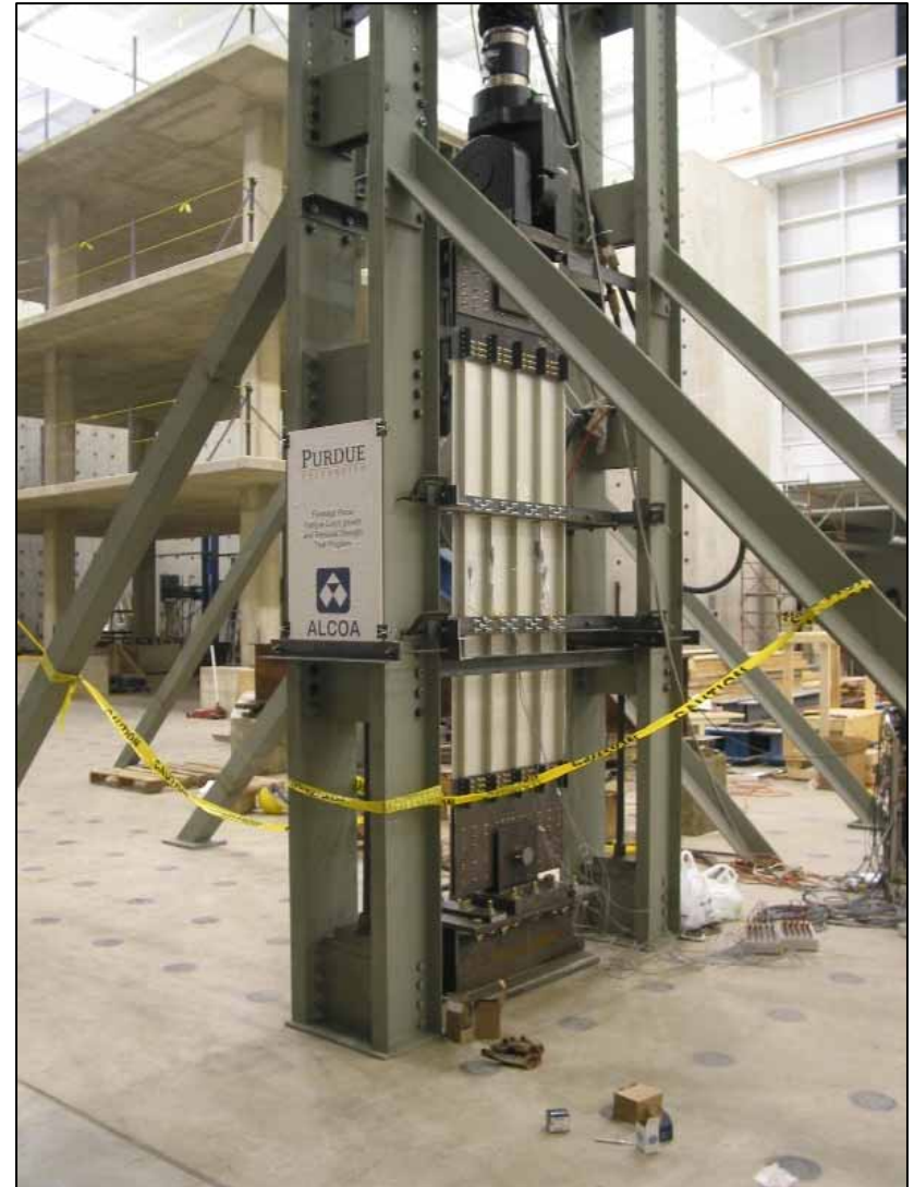
Fuselage crown stringer panel test set-up
