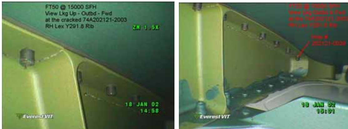
Figure 8 – Leading Edge Extension (LEX) cracks at 15,000 SFH
