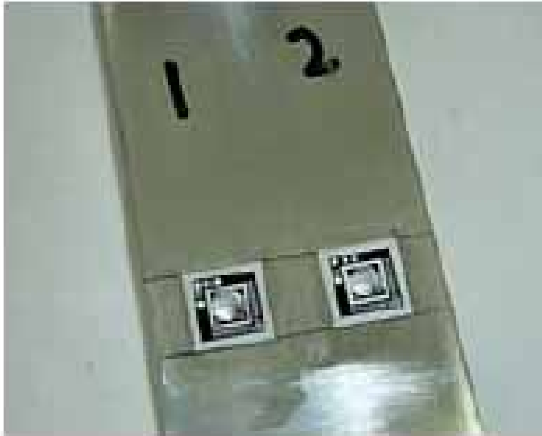
Figure 12. Fatigue test coupon with DMI gages
