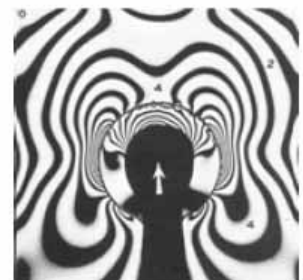
FIGURE 12. Pin in the Hole of Plate Loaded by a Force on the Pin
