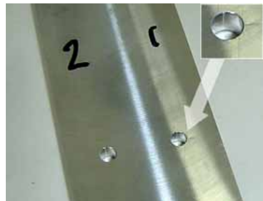
FIGURE 16. Crack location on back side of gage 24.
