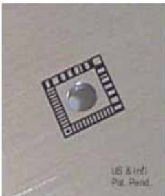
DMI Proprietary Gage Centered On Open Hole
