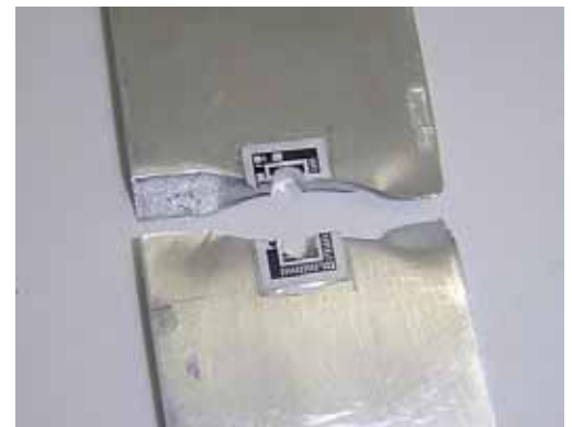
FIGURE 19 Fatigue Coupon after failure
