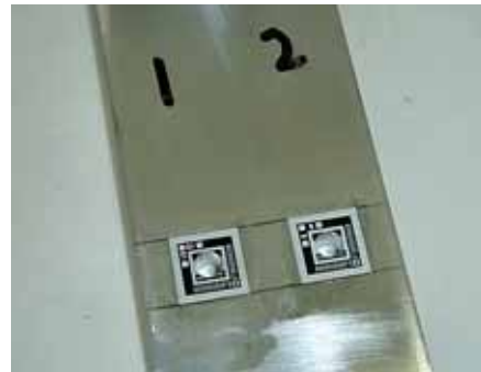
FIGURE 13. Fatigue test coupon with DMI
