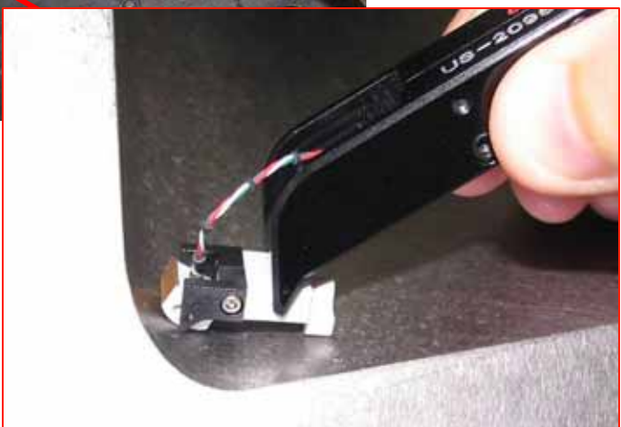
Pivot maintains coil compliance to inspection surface
