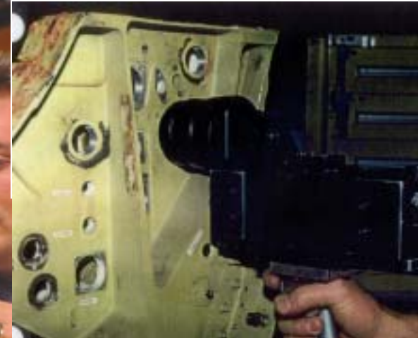
Cold expansion of non-circular holes
