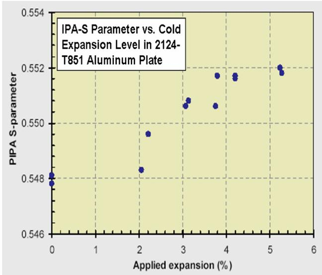
**Figure 9 – IPA-S Response to Cold Expansion in 2124-T851 Plates**
