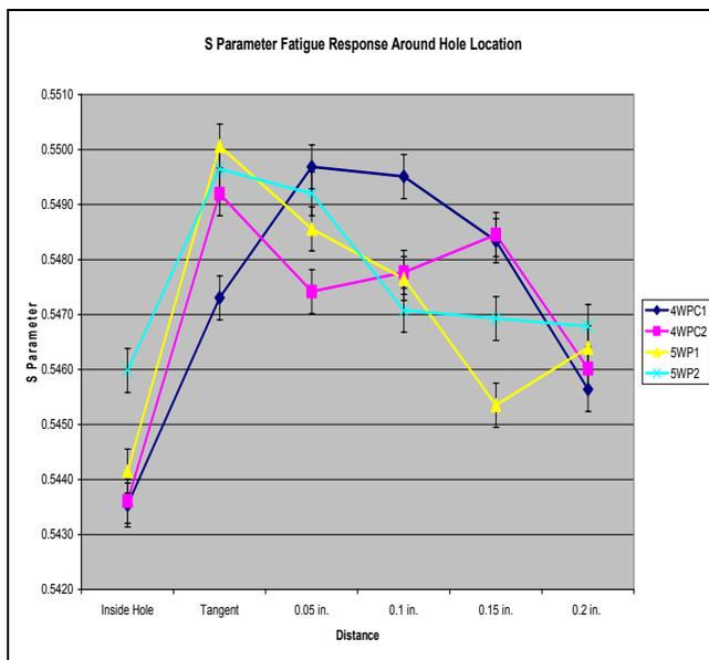
**Figure 10 - IPA-S Surface Residual Stress Distribution around Cold Expanded Hole**
