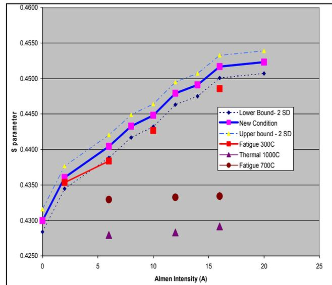
**Figure 6 – IPA-S Near-Surface Shot Peening Response and Thermal and Mechanical Effects on Surface Residual Stress**
